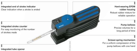
Integrated tube opener Simple scoring of the tubes using a ceramic blade for clean opening
